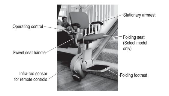
**Folding Footrest:** The footrest can be folded up and out of the way when the lift is not in use. The footrest must be in the down position when riding the lift. Sensors are provided in the footrest to detect obstructions. When an obstruction is encountered, the lift will stop. The obstruction must be removed to move the lift.
