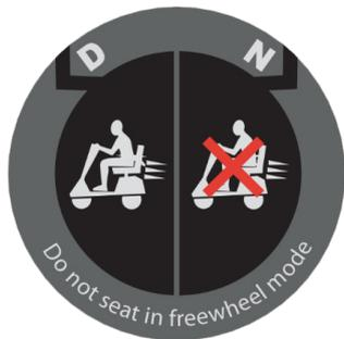
Place unit on level ground when changing from “D” drive mode to “N” freewheel mode or freewheel mode to drive mode.
