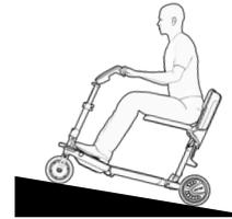
Do not try to descend or climb an incline with an angle greater than recommended. See the "Specifications" section of this Owner's Manual.
